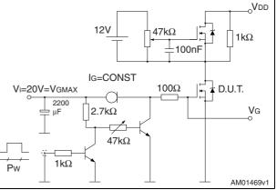
Gate charge test circuit
